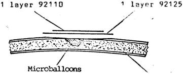
core made of Copticell
